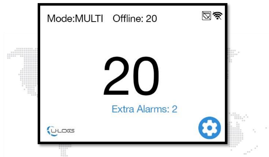
Figure- 5 Main screen displaying the total number of detected security tags
